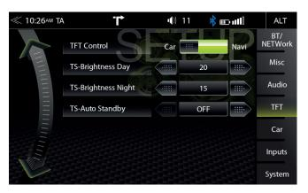
In the TFT Setup menu you can make screen settings that control the day/night brightness of the TFT LCD display screen. This will only work with microSD card from the ZENEC navigation software bundle (Z-E3756-SDFEU).
