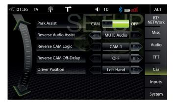
In the Car Setup menu, you can set how the ZENEC device interacts with optional components such as cameras and parking assist inside the vehicle. In addition, it can be defined whether the vehicle is a right or left-hand drive model.
