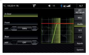
In this Expert Mode menu, you can adjust the High-pass transition frequencies of the front and rear speakers. The factory default is OFF for front and rear speakers.
