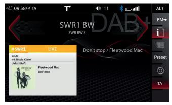
The DAB+ source menu offers a control- + operating section on the right side of the display, allowing for simple and convenient direct adjustments of DAB+ functions in the playback menu.
