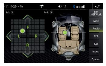
In this Expert Mode menu page, you can adjust the balance and fader. Press and hold the green dot of the crosshair to move sound center position into any desired position.
