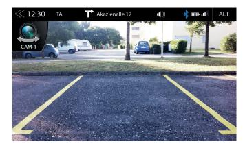
Tapping the camera icon starts the manual camera mode, when a CVBS type camera is connected to the camera input of the unit.
