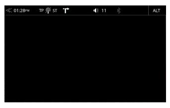
The "info bar" in the upper hand screen area shows TA, volume and time but also contains two important controls for device operation: BACK (left side) and ALT (right side).
