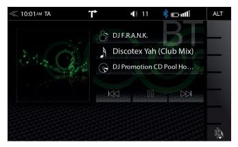
The A2DP RVC interface offers Play, Pause and Skip control of previously paired smartphones in audio playback mode. The iD3-Tag meta data display is possible only when tag data is contained in the streamed music track.
