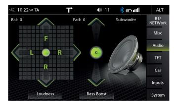
In this menu, you can adjust the Balance / Fader, Loudness, Bass Boost and Subwoofer level of the speakers in the vehicle.
