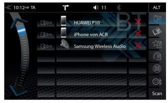
The BT function on the device must be activated to invoke connection process. Please pay attention to the smartphone manufacturer's instructions regarding device pairing.
