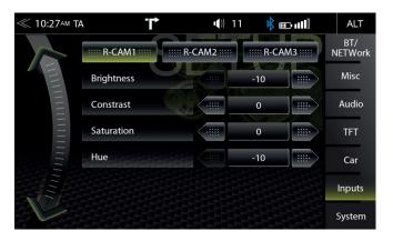
In the Input Setup menu, you can adjust the image settings of each connected camera channel, such as reverse cameras. Contrast, brightness, color saturation and hue can be adjusted.
