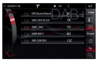
Once the first DAB+ band scan has completed, device will show all DAB+ Ensembles and radio stations of sufficient signal strength. The Ensemble list and its content is auto updated periodically.
