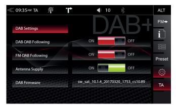
The setup page for the DAB+ tuner allows to define important functions such as DAB<>DAB and FM<>DAB station following. And also to activate the phantom power supply voltage of the DAB antenna socket.
