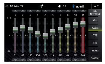
In this Expert Mode menu page, you can set the 10-Band graphical equalizer. Press and hold the individual band level sliders to move it up or down for a level change.
