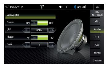
In this Expert Mode menu, you can adjust Phase, Gain, and Low-pass transition frequencies of the subwoofer. The default settings are Phase 0°, Power ON, LPF 100 Hz.
