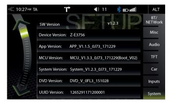
In the System Setup menu page under SW version, you will see the currently installed software versions with detailed version info for MCU, OS and APP etc., including a simple Short Software Version.
