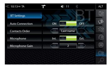
On the Bluetooth setup page you can adjust settings for Bluetooth operation. Press the appropriate button / field to change any of the listed settings.
