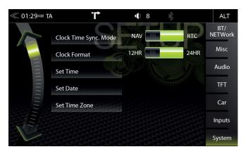
In the System Setup menu page under Clock & Date, you can set the format, change the displayed time and select the time sync source (system time or GPS) for the time display.
