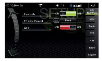
In BT / Network Setup, you can make important changes for best Bluetooth operation. Tap on the ON / OFF button of desired field to effect a change.
