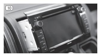
Connect all the cables to the ZENEC system (No. 1): those previously run in the radio slot, and the original antenna cable. If necessary, use the ISO DIN antenna adapter (No. 8) included in the kit.
