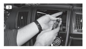
3. Remove the two original Torx screws at the top (T25).
