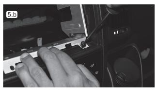
5.b Screw down the mounting frame at the top and bottom with the four Phillips screws (No. 3) supplied with the ZENEC system kit.
