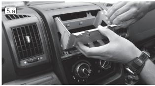
5.a Insert the mounting frame (No. 2) at an angle from above into the radio slot.
