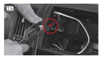
2.b Use a suitable saw to do this, and then a file to remove any protrusions still present.
